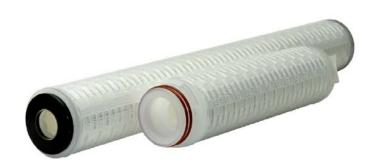
The Bioflo NY filter element is manufactured using a highly positive charged, Nylon 6.6 membrane, its Zeta potential retains negatively charged fine particles even smaller than the pores size itself.
